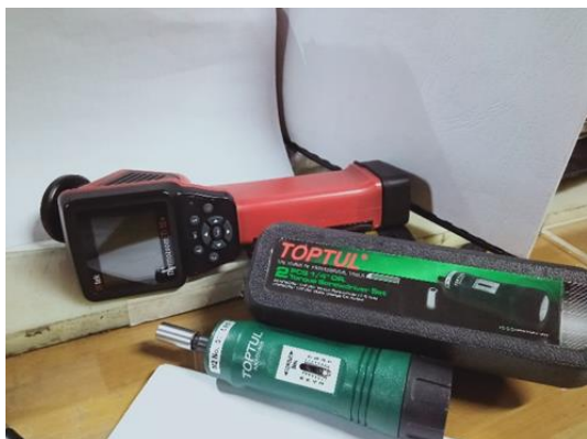
Figure 5. IR Thermograph and Variable Torque Wrench
